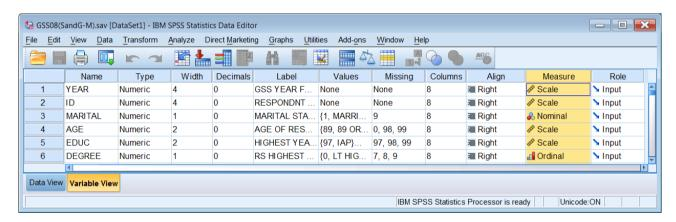
Click and hold down the left mouse button on **Measure** to drag it to the new position after **Name**: a thin vertical red line indicates the destination currently reached.
